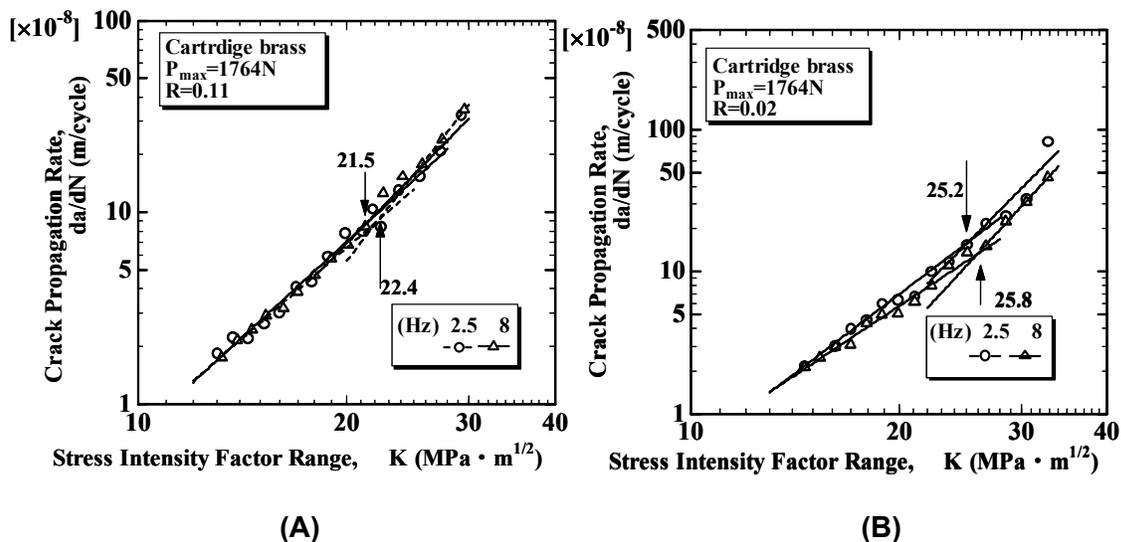
Fig. 3 The transition points at 2.5Hz and 8Hz, (A) with R of 0.11, and (B) with R of 0.02.
