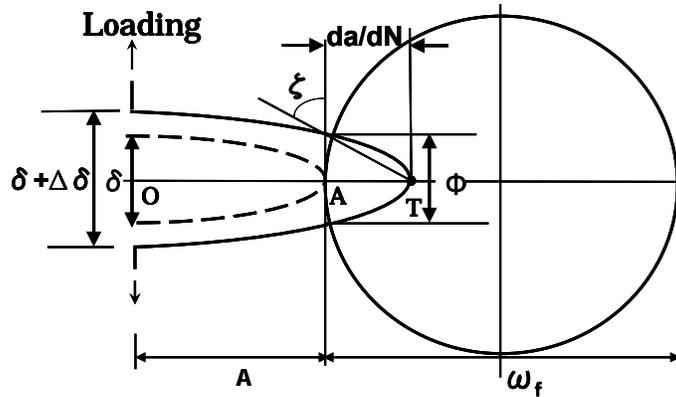
Fig.1 Schematic illustration of opening fatigue crack
