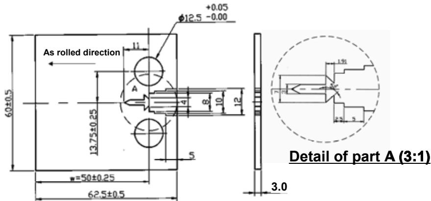
Fig.2 Illustration of CT specimen
