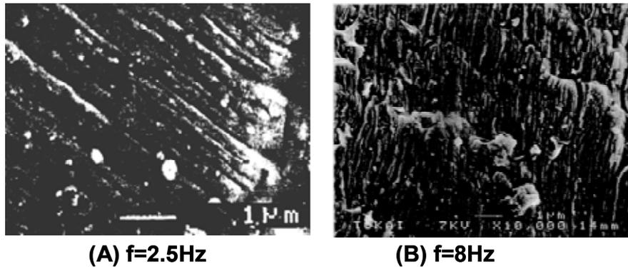
Fig.7 Striations formed on fatigue fracture surface of cartridge brass with R of 0.02.
