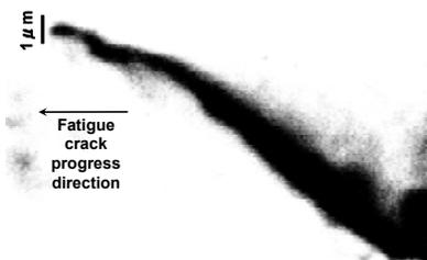
Fig.6 Crack tip at length of crack around 17mm.
