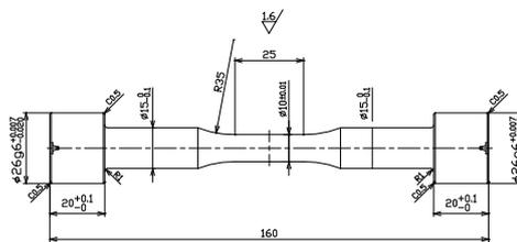
Fig.2 Geometry of fatigue specimen
