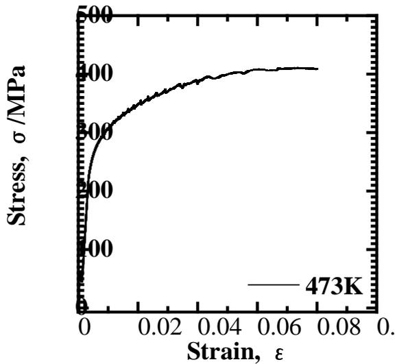
Fig.4. Stress - Strain curve at 473K
