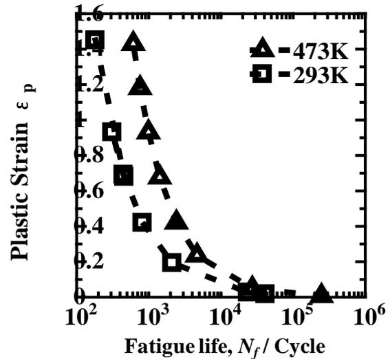
Fi.6 Diagram Plastic strain vs. Fatigue life
